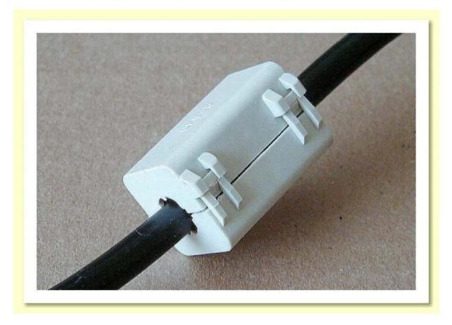
The photo above shows a typical device. It consists of a block of ferrite material that can be clamped around a mains cable and surround a section of the cable. This means it is exposed to the Electromagnetic (E and H) fields around the cable.
